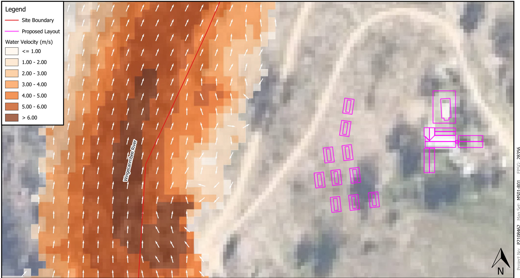
PMF Existing Condition Water Velocity (m/s) - Community 1
